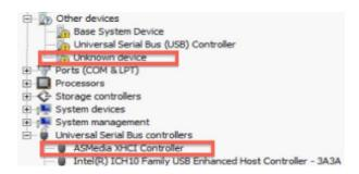
This '**Unknown device**' is the USB Hub device that is associated with each port. Repeat the above prove of right-clicking the '**Unknown device**' and point it back to the same folder location.
