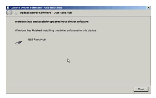
You will now have a 'USB Root Hub' device, simply right-click on the remaining 'Universal Serial Bus (USB) Controller' and select 'Scan for hardware changes', the required drivers will be installed. Many drivers will be shown as installing; once the process finishes you will still be left with a 'Base System Device' in 'Other devices'. There is no driver available to resolve this, however it should not impact the overall card working.
