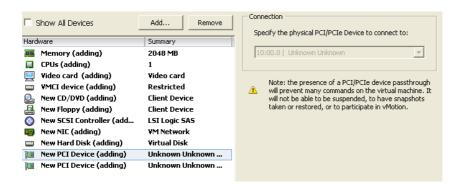
Once you have a fully installed Windows 7 machine, log in and follow steps 2, 3, 4, 5, 6 and 7 from the Windows 2008 R2 installation section and you should end up with 2 x dual bay devices showing  $4 \times 3TB$  drives connected to your virtual machine
