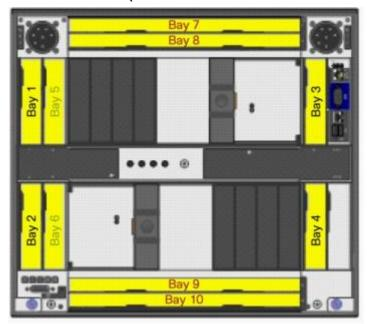
There's roughly 10 firmware items to flash on each blade, and up to 10 switch modules in back of the chassis to also flash, that's a lot to handle!
